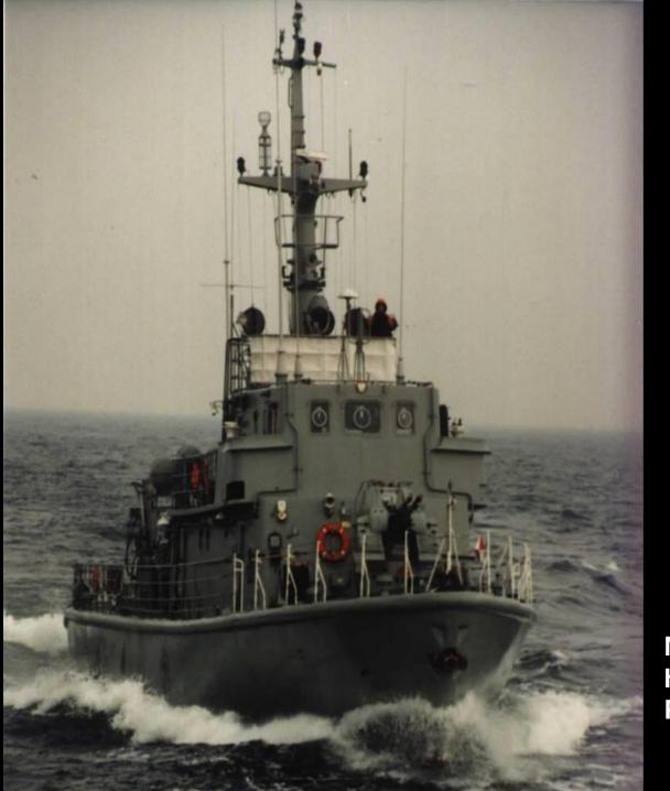
Mine-sweeper – hull made of GRP – Polish Navy
