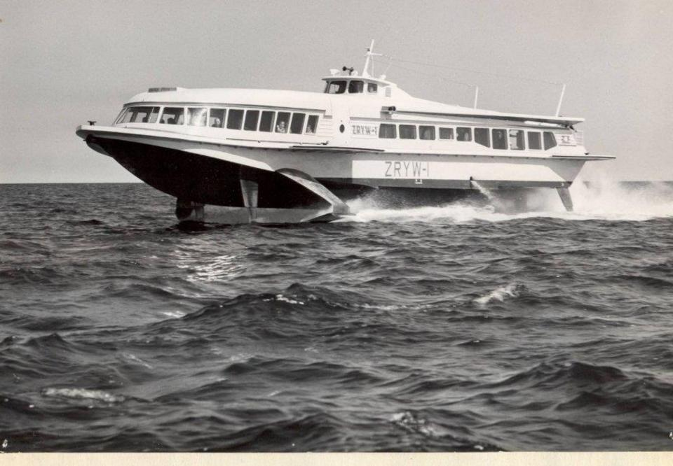
"ZRYW" - Hydrofoil – sea going vehicle (L=27.6m; speed 35 knots=65 km/h) designed by the Faculty of Ocean Engineering and Ship Technology, GUT
