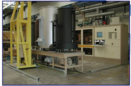
Laboratory equipment for CVD coatings deposition (*Ion Bond*)
