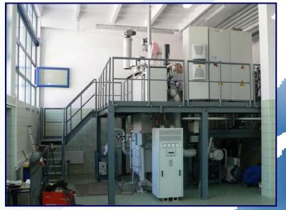
Laboratory vacuum furnace for directional crystallization of nickel base alloys (ALD)
