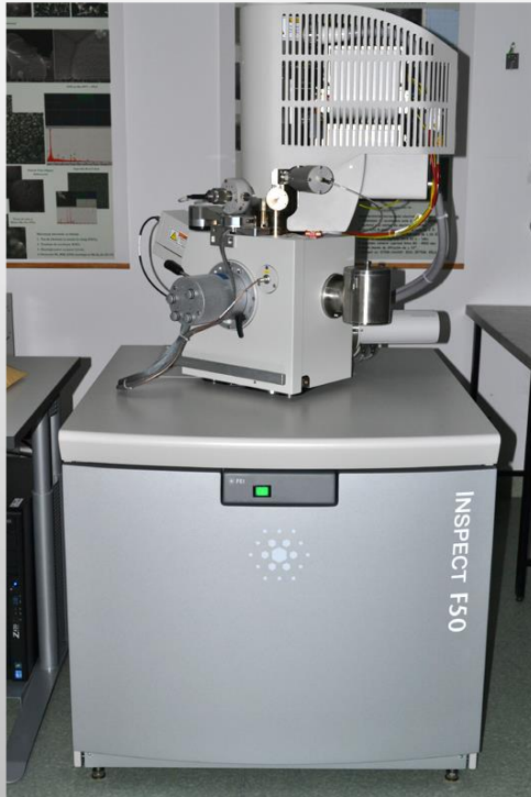
Scanning electronic microscope for high resolution imaging
